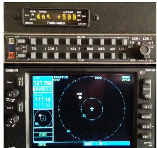
Thanks to its compact size the ATD-300 can be located anywhere in the panel. Connect to the audio panel and the navigator display for total traffic awareness. Mounting brackets and connectors are provided with the unit.
