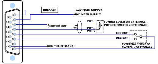
15-pole female connector, view from wiring side
